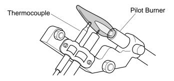
Figure 19 - Correct Pilot Flame Pattern
